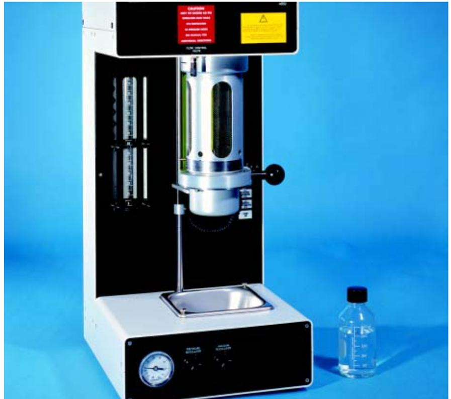
The HIAC Model ABS-2 is a pressure sampling device used for batch analysis of volatile or viscous fluids. The Model ABS-2 accurately delivers fluid to the sensor at flow rates of 10 to 200 mL/min. It contains a precision metering valve for accurate control of flow rates, regardless of sample viscosity. A check valve in the sample introduction line eliminates backflow and minimizes sample cross contamination, and an automatic drain mechanism allows unattended sample analysis of multiple runs.
