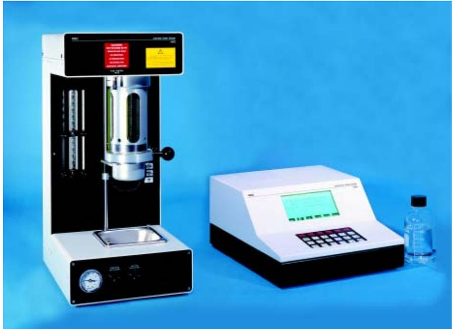
The HIAC Model 8011 liquid particle counting system provides immediate particle concentration data for low and high viscosity fluids. Composed of a light blocking or dual mode sensor, the Model 8011 system pressurizes fluid in an ABS-2 (Automatic Bottle Sampler) for precise volumetric sampling of industrial fluids.
