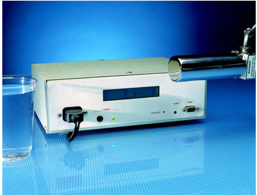
The HIAC Model 2000 provides an accurate yet inexpensive means to transfer particle data from sensor to host computer system. Up to four channels of particle size information are available. The instrument is constructed of corrosion-resistant anodized aluminum for placement in non-laboratory environments. A liquid crystal display allows the operator to view the data at the analysis site for real-time observation and decision making.
