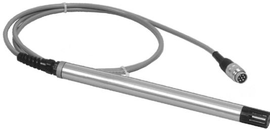
RH/Temp Probe – P/N 2080245-1. Plugs into the connector on rear of unit. The probe monitors relative humidity (10% to 90%) and temperature (5 to 125°F, or -15 to 50°C). The particle counter displays the reading and includes it in the internal particle count data record.
