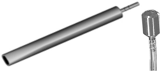
Isokinetic Probes – Wand style P/N 203015-3, Direct mount P/N 2080613. For use in laminar air flow up to 100 feet per minute. The probe is used by facing the open end into the direction of the air stream.
